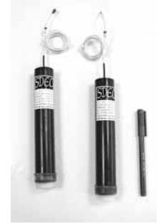
SENSOR PLACED ON THE TENSIOMETER TUBE for PERMANENT installation
